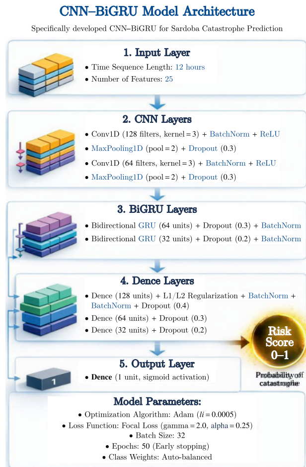
Figure 3. Architecture of the proposed CNN–BiGRU framework for dam failure risk early warning, illustrating convolutional temporal feature extraction, bidirectional recurrent sequence modeling, and probabilistic risk estimation
