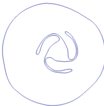
Figure 10. Cross section of the balloon compared with the undeployed configuration
